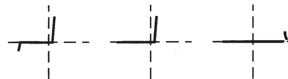
Typ: NPN-Transistor Pole: B-E B-C E-C Anschlüsse:(CT - Masse) (CT - Masse) (CT - Masse)
